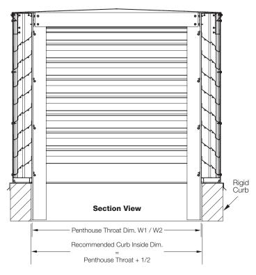
**Recommended Sizing:** (For optimum performance W1 and W2 should be  $\geq$  H  $\times$  2)
