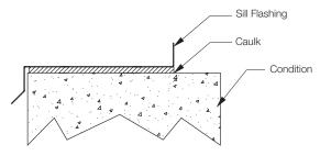
Figure 1.2 Sill Flashing Assembly
