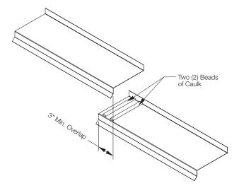
Figure 1.3 Closed End Sill Flashing
