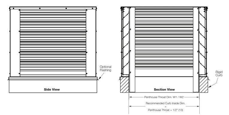
**Recommended Sizing:** (For optimum performance W1 and W2 should be  $\ge$  H  $\times$  2)
