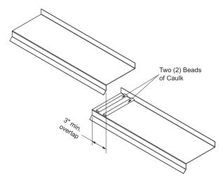
Figure 1.3: Closed End Sill Flashing
