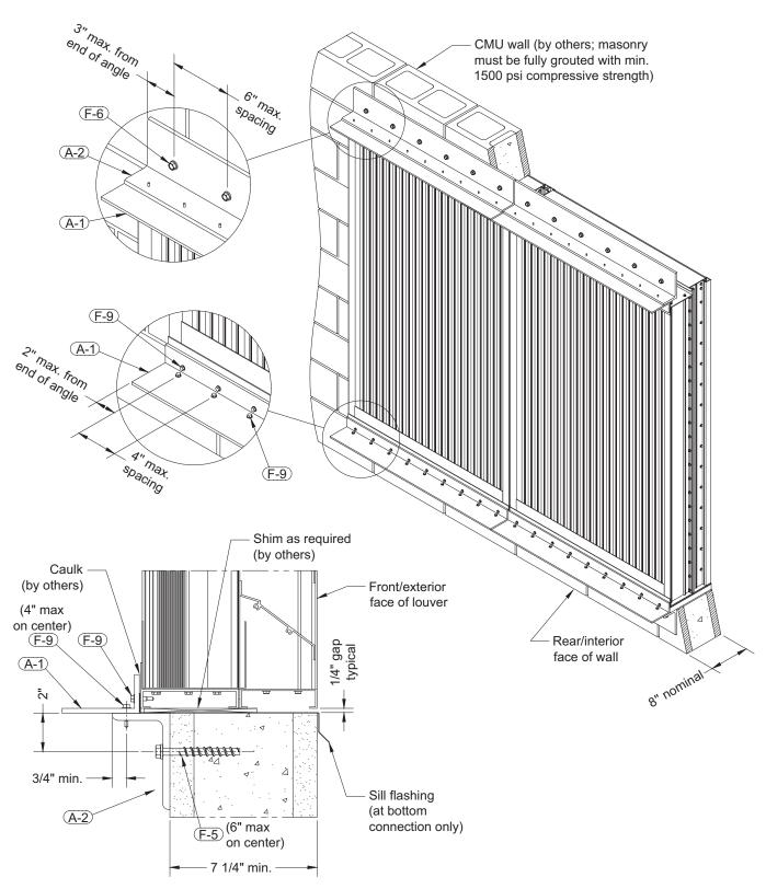
**Section Detail at Bottom Connection**
