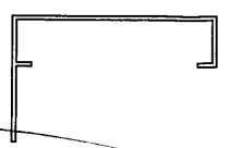
FLANGED JAMB, EFJ-437 SCALE 1:4
